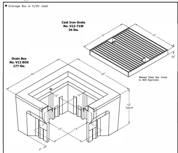
A high density reinforced concrete box with cast in galvanized frame, specifically engineered for heavy traffic areas. Approximate dimensions and weight shown.
